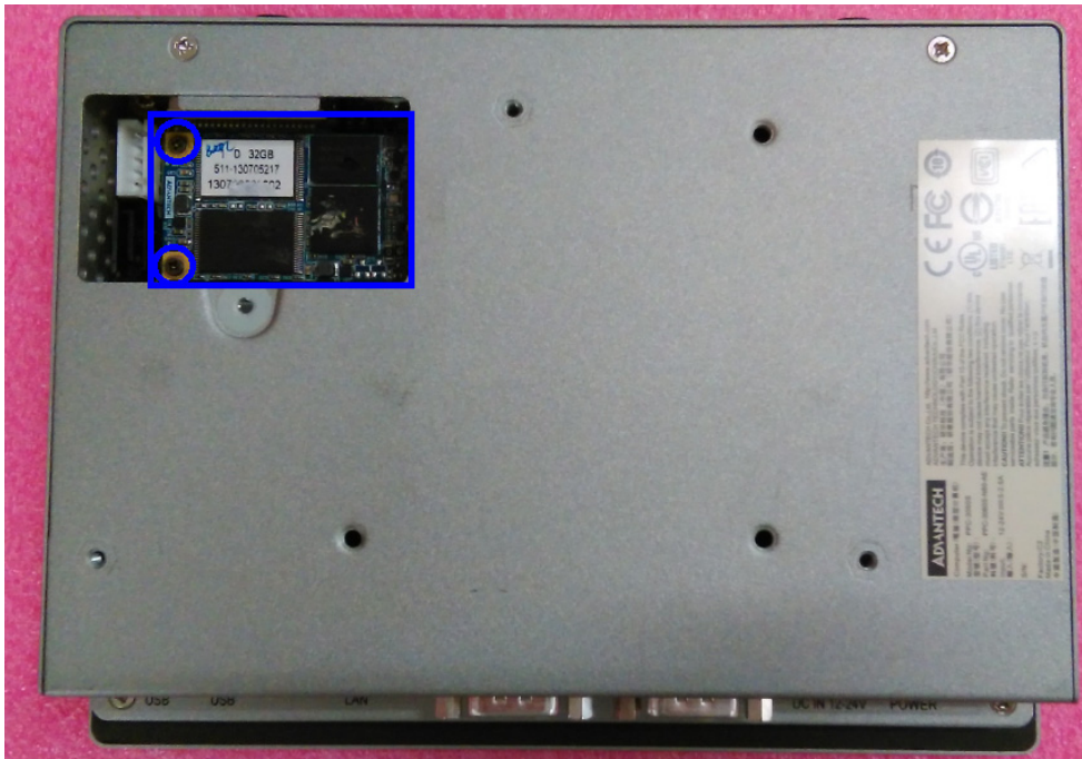
Figure 2.14 Installing the mSATA Module
