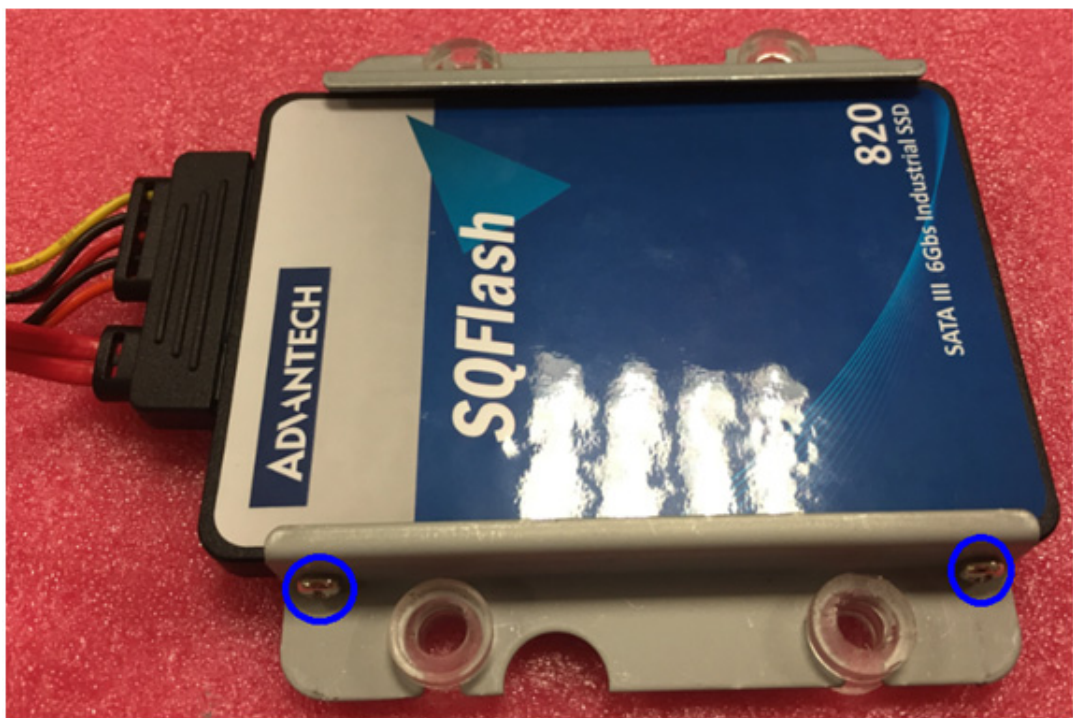
Figure 2.9 Connection of Cable and SATA HDD
